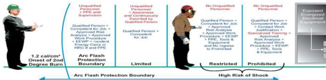
CSA Z462 Table 1 / NFPA 70E Table 130.2 (C) Approach Boundaries to Energized Electrical Conductors or Circuit Parts for Shock Protection
